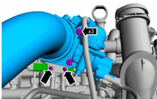
Install position sensor camshaft (CMP)
